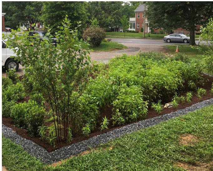
▲ **Green Infrastructure:** Rain garden and landscaping that work to reduce flooding and pollution caused by stormwater.
